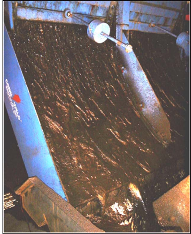
FIGURE 6 Production-scale sieve bend for fine coal sizing. Courtesy of Conn-Weld Industries.
