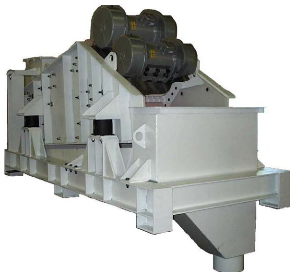
FIGURE 4 Production-scale high frequency screen. Courtesy of Innovative Screen Technologies.
