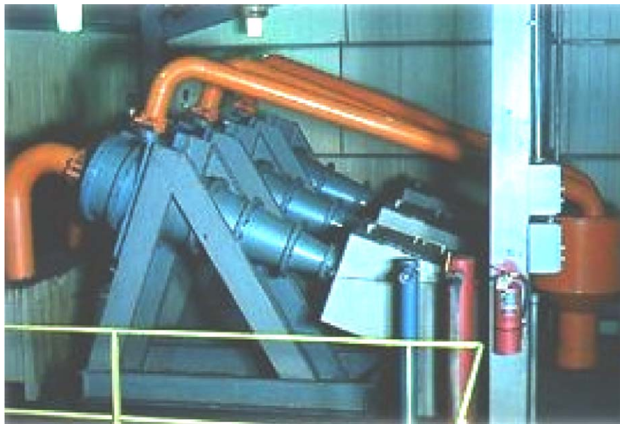
FIGURE 13 Illustration of a heavy media cyclone bank. Courtesy of Krebs Engineers.
